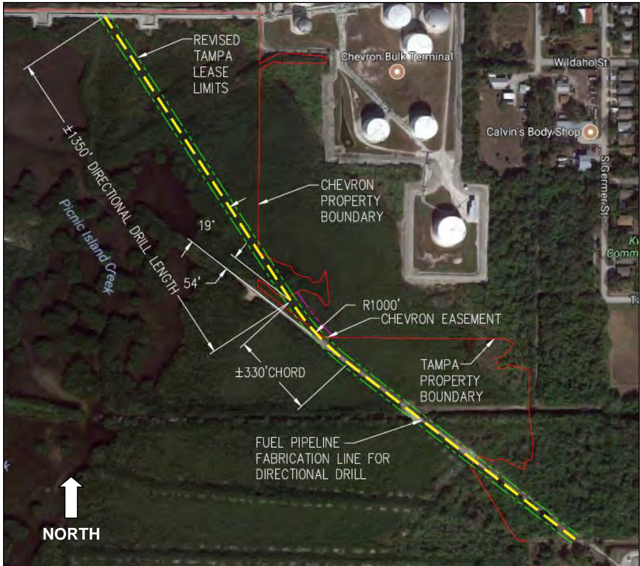
Figure 2-5. Aerial of Replacement Using Horizontal Directional Drill
